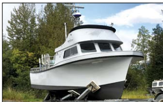
P2349M – 40' X 11' FIBERGLASS GILLNETTER, 975 HOURS ON 480 HP VOLVO TAMD 74 WITH TWIN DISC GEAR, TROLL VALVE, EXTENSIVE OVERHAUL IN 2010 INCLUDING; NEW INTERIOR, WIRING, FUEL AND HYDRAULIC LINES, ELECTRONICS, AUTOPILOT, LED LIGHTING, 2 EA. 225 GAL. FUEL TANKS, AFT DECKS, FISHHOLDS, CABIN ROOF, WINDOWS, DOOR, RAISED BULWARKS, AMERON EPOXY HULL COATING. 18 KTS, CRUISE 22 KTS MAX, PACKS 13K. VERY CLEAN AND TURN KEY. ASKING $270K.
