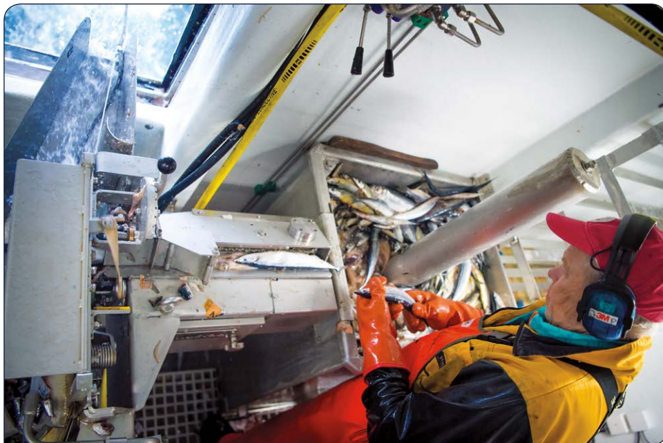
Mustad Autoline says its systems can bait up to 80,000 hooks per day, with a successful baiting rate of 95 to 97 percent. Photo courtesy of Mustad Autoline
