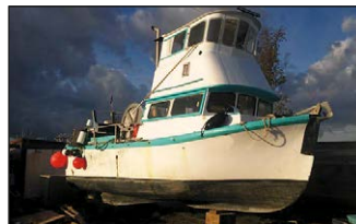
P2280M – 32 X 13 RSW FIBERGLASS TOPHOUSE STERNPICKER, TWIN IZUSU MAINS, BORG WARNER GEARS. PACKS 23K UNDER DECKS IN 11 HATCHES. 5 SHACKLE SLIDING REEL W/ LEVEL WIND. NEW ANCHOR GEAR, GARMIN PLOTTER. NEW LED DECK LIGHTS AND FORWARD LITE BAR. NEW IN 2017 GLENN DENNING ELECTRIC CONTROLS. NEW IN 2018: NEW DECKS/7.5 TON IMS RSW/4.8 CUBE HYDRAULIC PUMP AND TANK. NOW HAS TWO SEPARATE SYSTEMS. NEW TRANSMISSION MOUNTS. TURN KEY W/3 SHACKLES OF GEAR. ASKING $125K.
